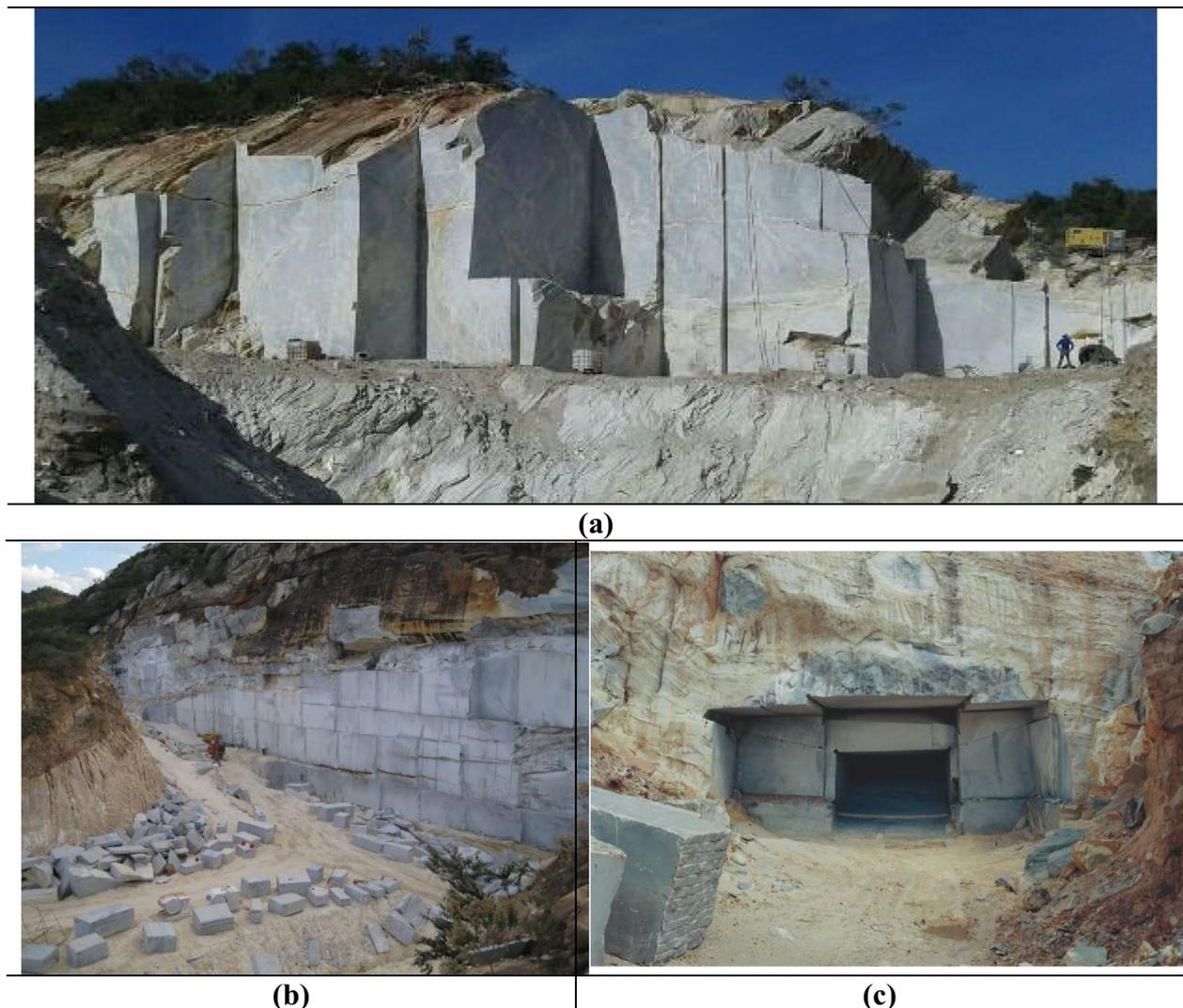
**Fig. 2** Some blue quartzite quarries (Bahia, Brazil). **a** ‘Imperial Blue’ quarry (Photo: Graniti Export); **b** ‘Blue Macaúba’s quarry (Photo: Blue Stones/GM Granitos e Mármore); **c** ‘Imperial Blue’ abandoned attempted underground quarry (Photo: Maria Heloisa Frascá)
