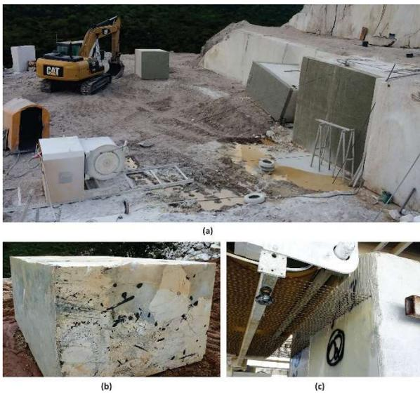
Fig. 3. Exotic stones production: quartzite quarry showing benches and blocks reinforcement (a); pegmatite block being reinforced at the quarry (b); and a multiwire saw cutting a reinforced quartzite block (c).
