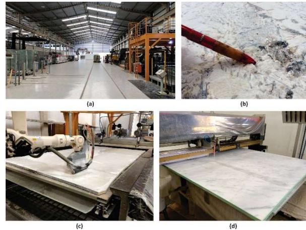
Fig. 4. Exotic stones production: automatized processing plant (a); cavities for filling (b); robotized resining for fibreglass fastening (c); automatic resin coating (d).
