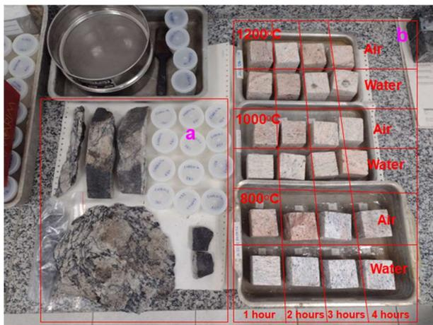
Figure 4: Samples in this study. a) Monument pieces of FAC and b) Cubic samples of LEP.
