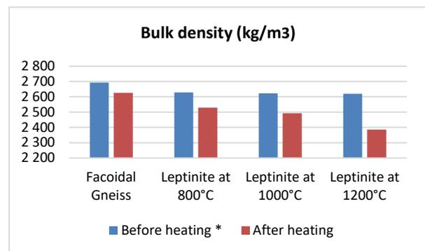
Figure 11: Bulk density of the samples before and after heating. \*FAC reference value from Castro et al., 2020.
