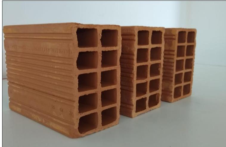
**Figure 2.** Sealing blocks with incorporation of 0%, 10% and 20% of wastes.
